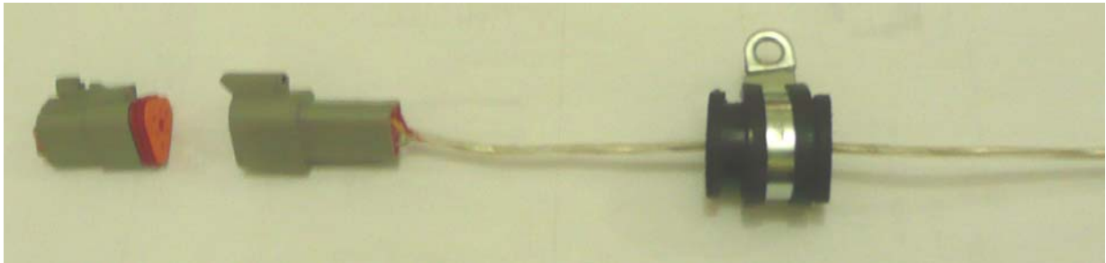
Photograph of Fire Wire with an end of line arrangement and clamping arrangement.
