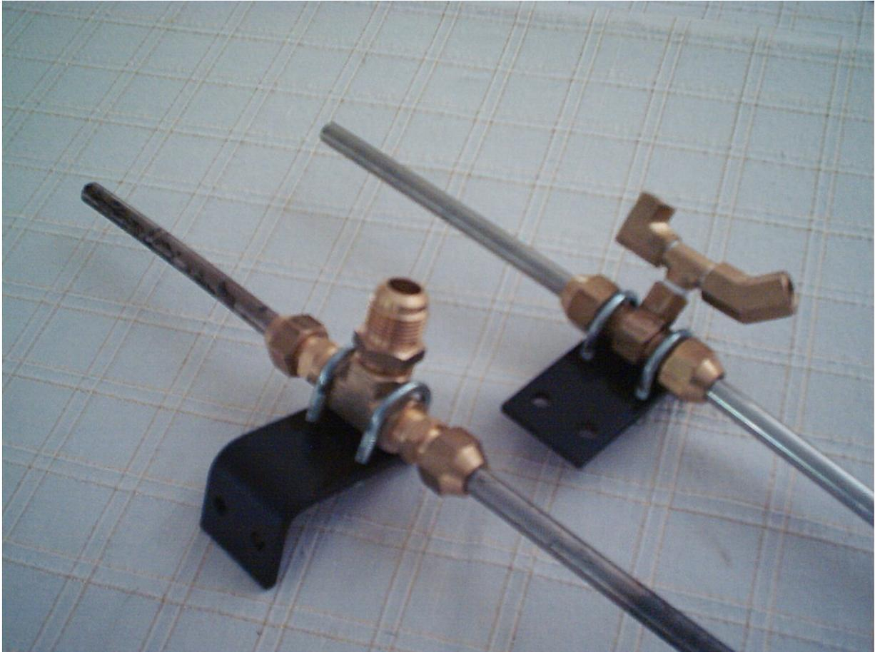
Photograph shows both brackets clamped to fittings
